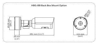
\* Dimensions drawing shows back box. Back box is compatible with a 4S electrical box.
